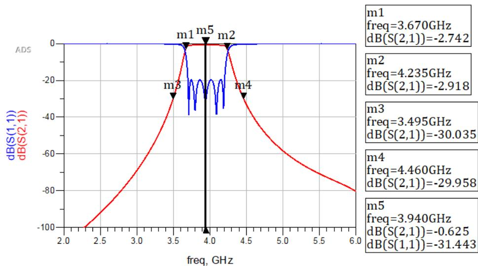
**Figure 9** The Optimized Result of the Fifth Order Parallel Coupled Line BPF
