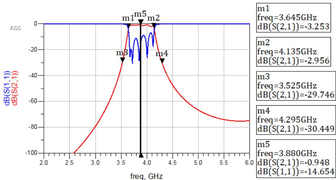
**Figure 5** Result of the Fifth Order Parallel Coupled Line BPF
