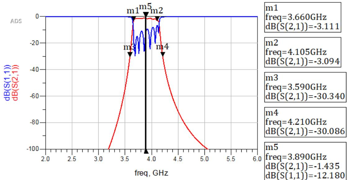
**Figure 7** Result of the Seventh Order Parallel Coupled Line BPF
