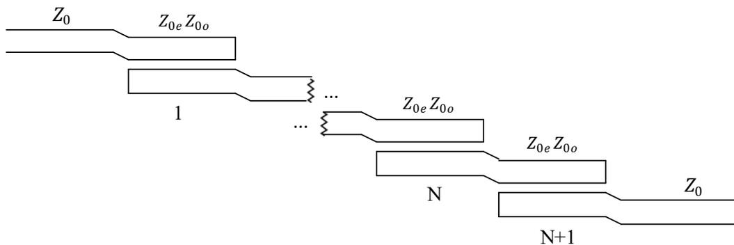
**Figure 1.** Layout for an  $N+1$  Section Coupled Line BPF
