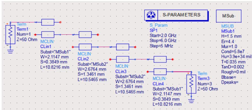
Figure 2 Schematic Diagram of the Third Order Parallel Coupled Line BPF
