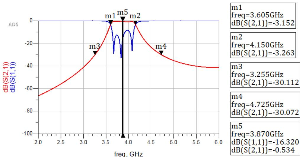
Figure 3 Result of the Third Order Parallel Coupled Line BPF
