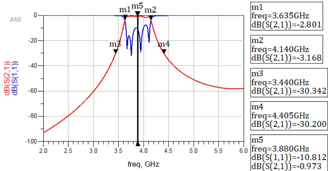
**Figure 4** Result of the Fourth Order Parallel Coupled Line BPF
