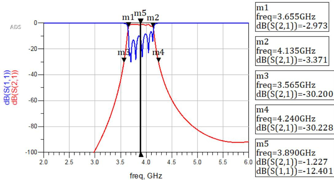
**Figure 6** Result of the Sixth Order Parallel Coupled Line BPF
