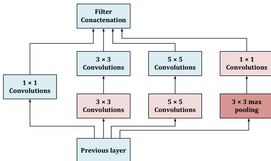
**Figure 2.** Block Diagram of the Inception V3 Module [14]
