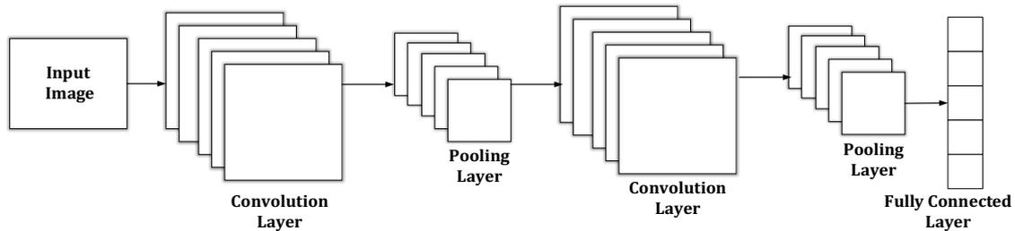
**Figure 1.** The Working Flow of the CNN Model
