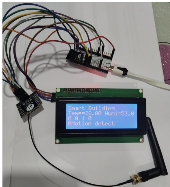
Figure 20. Experiment of motion sensor at remote building
