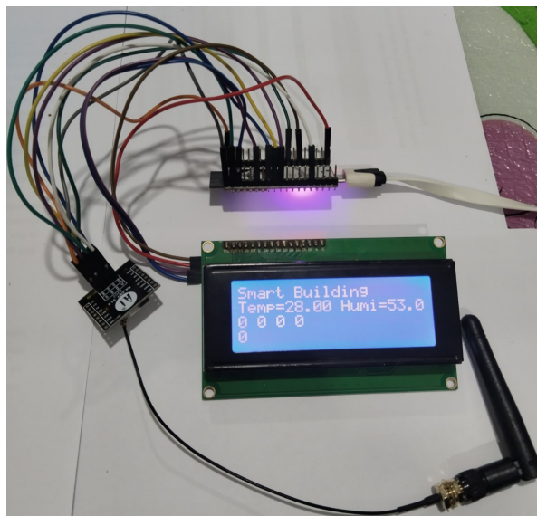
Figure 18. Experiment of temperature and humidity sensor at remote building
