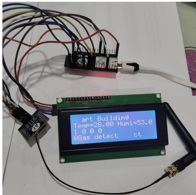
Figure 26. Experiment of gas sensor at remote building
