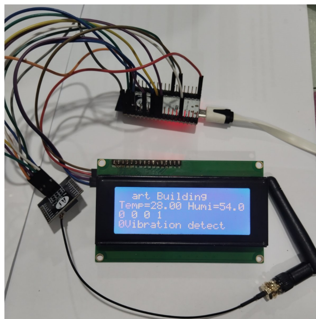
Figure 24. Experiment of vibration sensor at remote building
