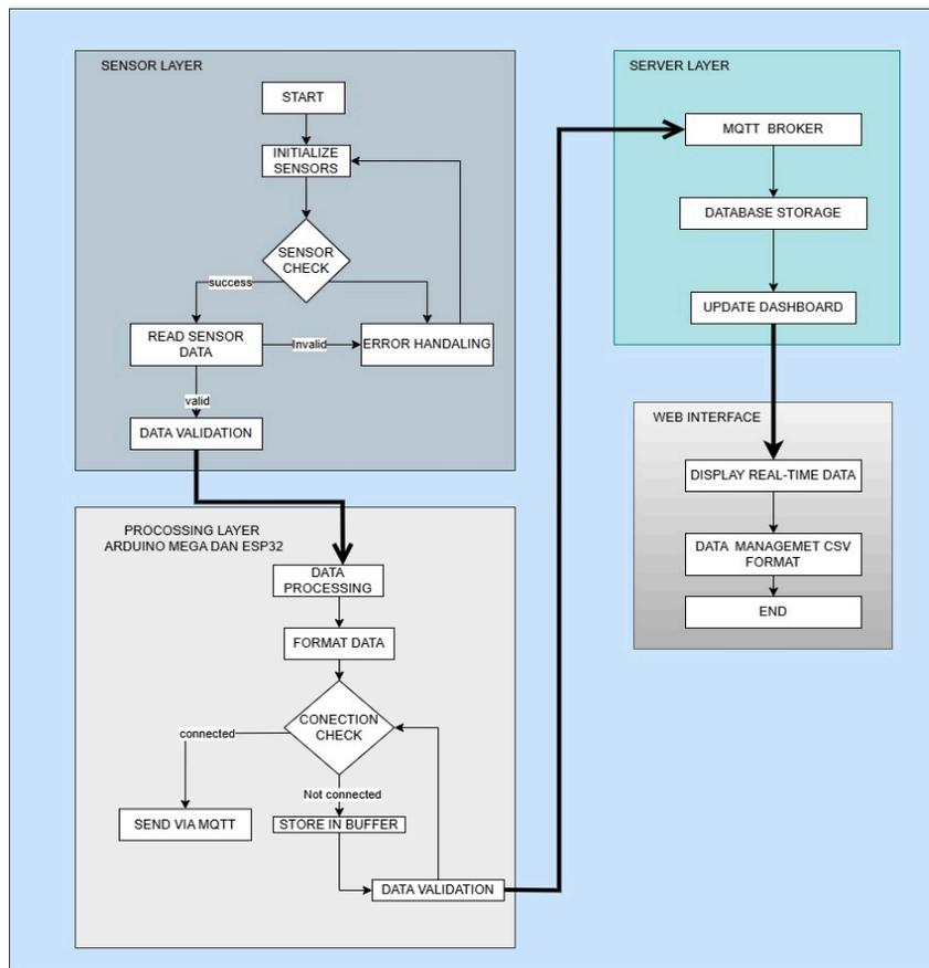
**Figure 2.** IoT System Architecture
