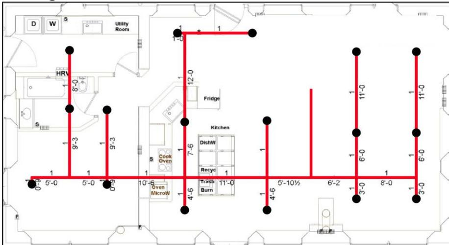
Figure 3. Input map#1 of the pipe network.
