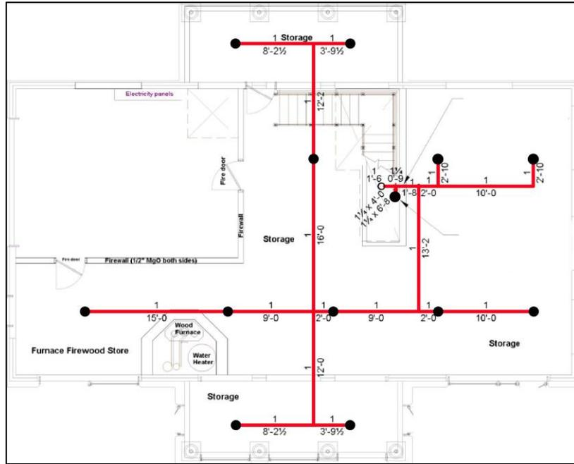
Figure 4. Input map#2 of the pipe network.
