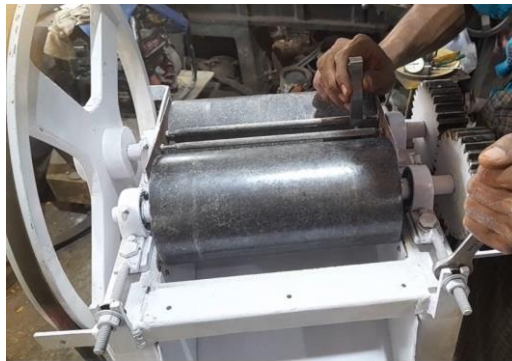
Figure 17. Construction of the Oat Flake Rolling Machine
