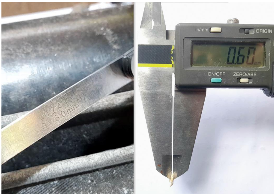
Figure 26. Roller Clearance for 0.6 mm Oat Flake Thickness
