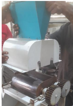
Figure 18. Assembling the Oat Flake Rolling Machine
