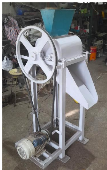
Figure 19. Assembly of Oat Flake Rolling Machine
