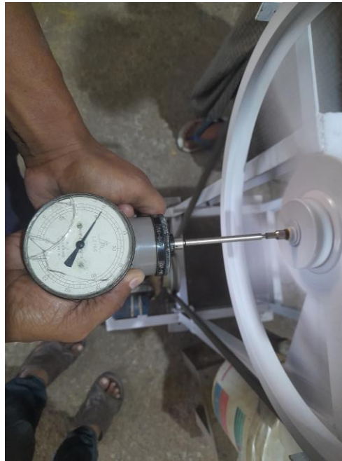
Figure 20. Measuring Speed with Tachometer
