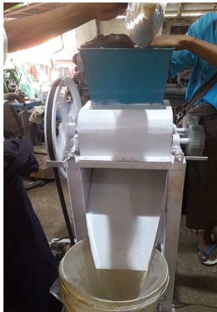
Figure 21. Processing the Oat Flake with Oat Flake Rolling Machine
