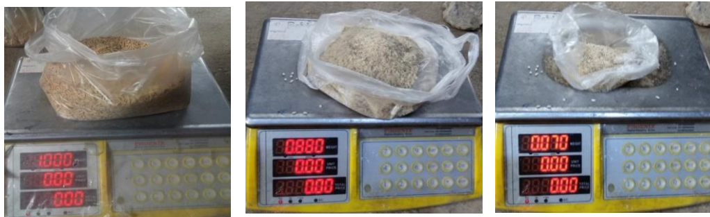
(a)Weight of paddy (b) Weight of well rice and weight of broken rice for modified blade
