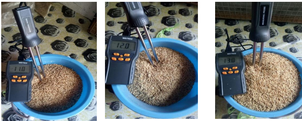
Figure 4. Moisture test for Ayayermin paddy
