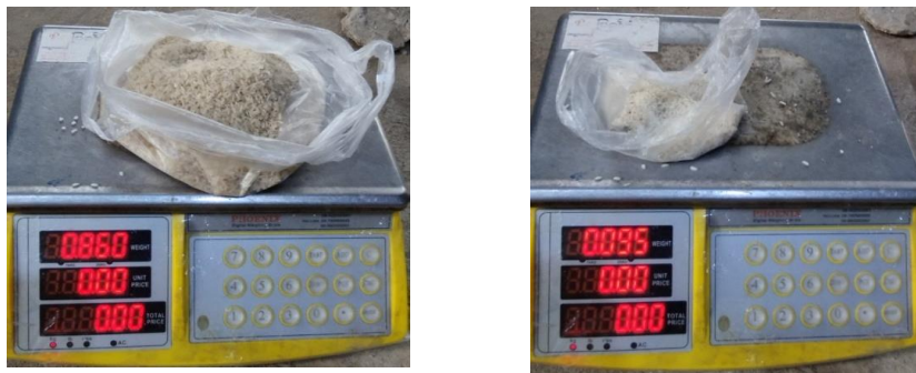
(c) Weight of well rice and weight of broken rice for existing blade
