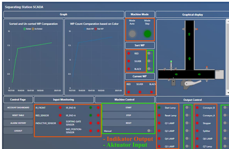
Gambar 5. Tampilan SCADA Separating Station 1
