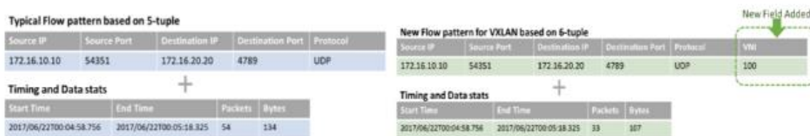
Figure 4 Typical flow pattern based on 5-tuple and new flow pattern for VXLAN based on 6-tuple
