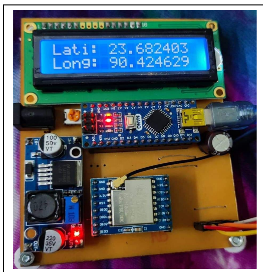
Figure 6. LoRa Receiver LCD display: longitude, latitude of LoRa
