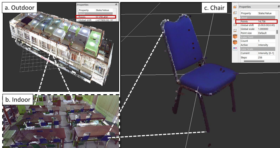
Figure 4. Scanning Results; (a) Outdoor Environment of Geodesy Building, (b) Indoor Environment, (c) Facility of Geodesy Environment Assets
